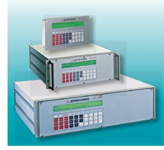
The DPC3000 is a multifunction dosing processor for all Engelhardt dosing systems. It is fitted with a bus system which places emphasis on its modular construction. Modules for the control of several vibrators, vibration belts and screw motors are at your disposal as well as programmable inputs and outputs for peripheral devices such as collecting or conveying systems and nesting units (coordination tables, turntables).
