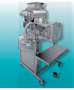
The gravimetric batch weighers of the series DW - T are dosing systems especially developed for mixing and difficult materials. Depending on the weigher type, the capacities are between 5g up to 5000g<sup>1)</sup> with 12 weighments/min and an accuracy up to 0.05%. As conveying systems belts, vibration channels, vibration belts or screw conveyors are at your disposal.
