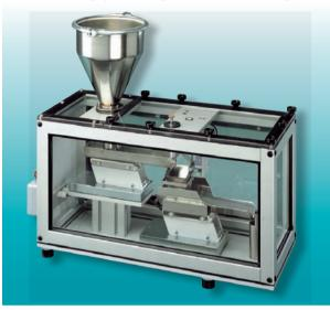
The gravimetric dosing weigher for small quantites KDW 0.1 is a continuous dosing system for granuals and free flowing powder.
