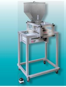
The gravimetric batch weighers of the series DW are newly developed discontinuous dosing systems for all kinds of bulk materials with batch weights between 5g up to 5000g<sup>1</sup>.
