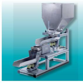
The gravimetric dosing weighers of the series KDW are newly developed continuous dosing systems for granuals, glass fibre and free flowing powder.
